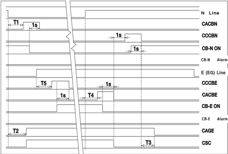
Switching sequence in the case of forced switching:
