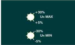
The minimum and maximum voltage thresholds are set using two of the trimmers set on the side of the device. The fixed maximum threshold is +5% and the fixed minimum threshold is -5% of the rated voltage.
