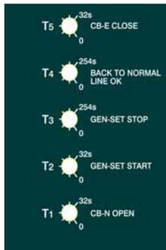
T1 Delay between net anomaly detection and opening of Normal line circuit breaker. Setting range: 0 to 32s. This avoids unwanted switching as a result of brief voltage drops.
